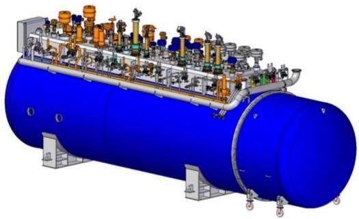
One Coldbox comprising 6 expansion turbines, 3 cold compressors, built-in acceptance test equipment Cold Box will arrive in site in mid 2017
